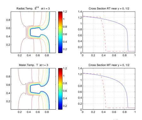
Figure 4.1: Contour levels and cross sections of the radiation temperature  $E^{1/4}$  and material temperature T at time t = 3 for  $Z_0 = 10$ . Contour levels:  $0.1, 0.2, \ldots, 1.2$ .
