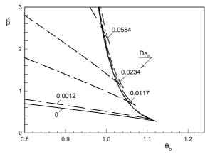
Figure 5 – Bifurcation sets for different values of  $Da_p$  (Da=0.0087,  $\gamma$ =21.8,  $D_e$ =2.79×10<sup>-10</sup> m<sup>2</sup>/s).
