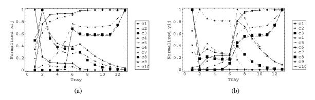
Figure 2: Normalized profiles of the liquid (a) and vapor (b) phase concentrations of one of the distillation columns.
