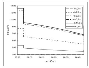
Figure 4b – Concentration profiles of PEG –3400 as function of time in the membrane.
