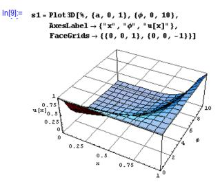
Out[9]= - SurfaceGraphics -Figure 4 – Sample 3D graph for first order reaction in slab geometry.
