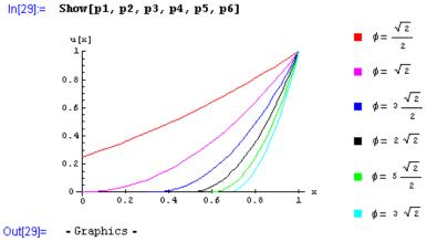
**Figure 3** –Positions of dead core for several values of  $\phi$ .
