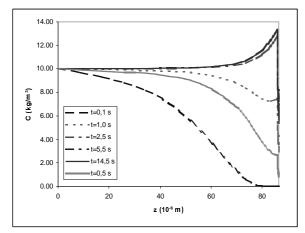
Figure 4a – Concentration profiles of PEG-3400 as a function of time in the polarization layer.
