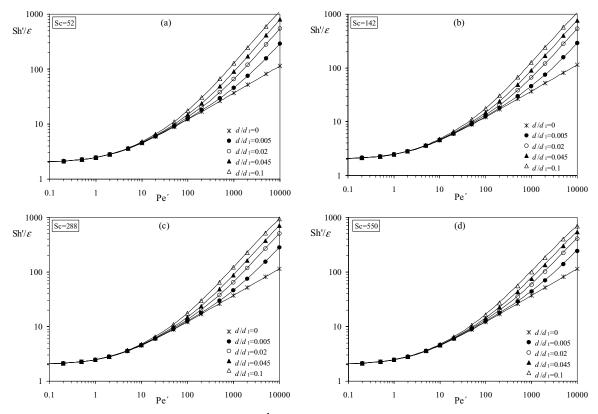
**Figure 2** - Dependence of Sh'/ $\varepsilon$  on Pe' for different values of  $d/d_1$  at (a)Sc = 52; (b) Sc = 142; (c) Sc = 288; (d) Sc = 550.
