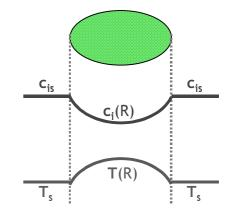
Figure 6. Concentration and temperature profiles in a non-isothermal catalyst.
