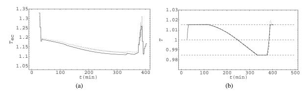
Figure 4: (a) Normalized inlet temperature jacket profile for (b) the optimal profile of the reactor temperature ( $\cdots$  PI; – MPC).
