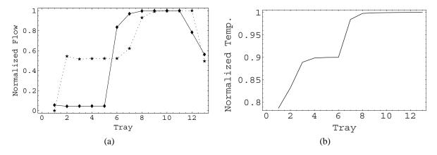
Figure 3: (a) Liquid (....) and vapor ( \_\_\_\_) phase flowrates and (b) temperature profile for one the distillation columns.
