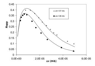
Figure 1 – Apparent rejection of PEG-3400 as function of the flux at two different circulation velocities. The predictions are the solid lines whereas the experimental data are presented by the symbols.
