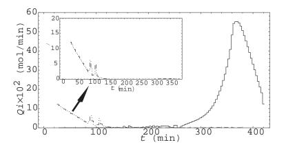
Figure 5: Optimal feed rate of initiators policy  $(-\cdots - \text{Kiparissides's model})$ , - Xie's model).
