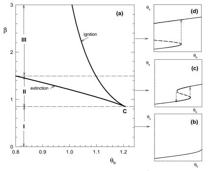
Figure 2 – Bifurcation set and bifurcation diagrams obtained for  $\lambda=0$  (Da=0.0087,  $\gamma=21.8$ ,  $\phi=0.76$ ).
