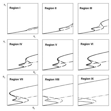
Figure 7 – Bifurcation diagrams obtained for *dc* model ( $\lambda$ =50), *d* model ( $\phi$ =0.7643) and *c* model (Da<sub>p</sub>=0.0117); (Da=0.0087,  $\gamma$ =21.8).
