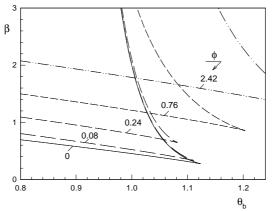
Figure 4 – Bifurcation sets for different values of  $\phi$  (Da=0.0087,  $\gamma$ =21.8).
