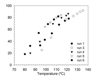
Figure 1 – MNB production as a function of the reaction temperature for runs 1, 3, 4, 5 and 6.
