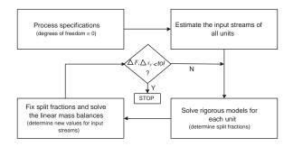
Figure 4: Schematic representation of the strategy for overall simulation of the purification stage.
