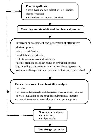
Figure 1. Strategy for designing chemical processes with good economic and environmental performance, using computer modeling and simulation
