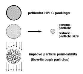
Figure 17 – How to decrease intraparticle mass transfer resistance?
