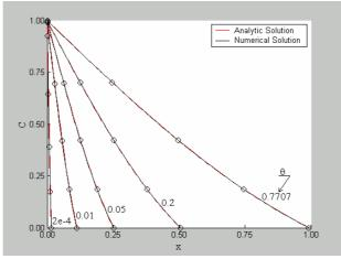
Figure 1: Concentration profiles in phase I for various values of  $\theta$
