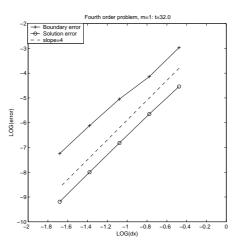
Figure 6: Order of accuracy in the  $L^1$  norm of an approximation to a onedimensional (d = 1) self-similar solution of the fourth order equation with m = 1.
