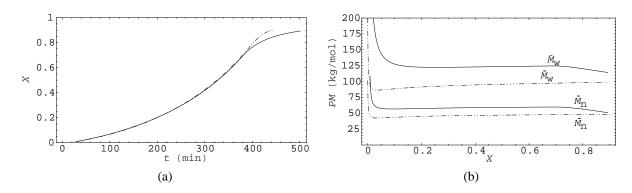
Figure 1: (a) Conversion profile for isothermal operation and (b) conversion dependence of number and weight average molecular weight  $(-\cdots - \text{Kiparissides's model})$ .
