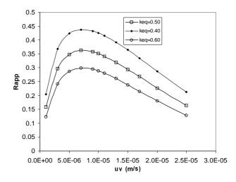
Figure 3 – Effect of equilibrium partition coefficient on the apparent rejection of PEG-3400
