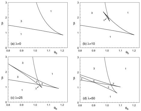
Figure 1 – Bifurcation sets for different values of  $\lambda$  (Da=0.0087,  $\gamma$ =21.8,  $\phi$ =0.76).
