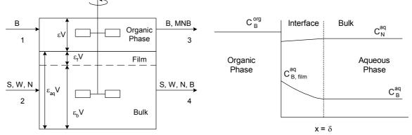
Figure 2 – Schematic representation of the film model in the pilot reactor.
