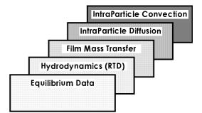
Figure 14. Factors governing the behavior of an adsorptive process
