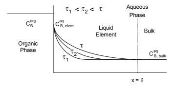
Figure 4 – Concentration profiles in the stagnant element as function of contact time – penetration model.
