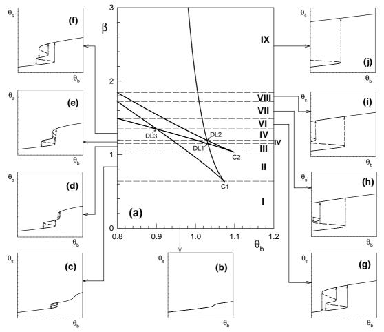
Figure 3 – Bifurcation set and bifurcation diagrams obtained for  $\lambda$ =50 (Da=0.0087,  $\gamma$ =21.8,  $\phi$ =0.76).
