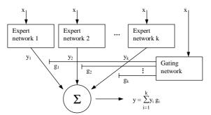
Fig. 1. Block diagram of a 'mixture of experts' network; the outputs of the expert networks are mediated by a gating network.
