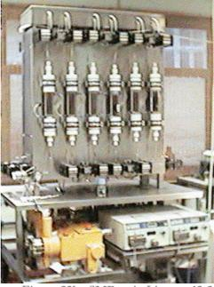
Figure 23b. SMB unit *Licosep 12-26* (Novasep) at the *LSRE*
