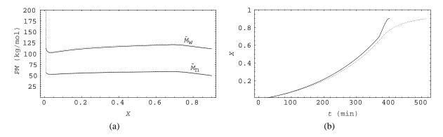
Figure 3: Comparison between the optimal and base profiles using Xie's model: (a) Average molecular weights and (b) conversion profiles ( $\cdots$  base case, – optimal).
