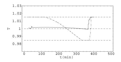
Figure 2: Normalized optimal reactor temperature policy  $(-\cdots - \text{Kiparissides's model})$ .
