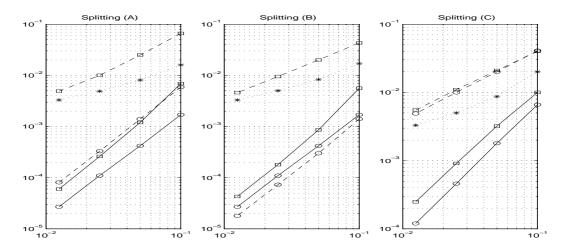
Fig. 3.6.  $L_2$ -errors versus  $\tau = h$  for the splittings (A), (B) and (C). Methods ROS1 (dashed lines) and ROS2 (solid lines) with  $\theta = \frac{1}{2}$  (circles) and  $\theta = 1$  (squares). Results for Yanenko's method are indicated with stars.
