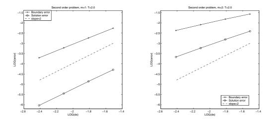
Figure 2: Orders of accuracy in the  $L^1$  norm of approximations to onedimensional self-similar solutions of the PME for m = 1,  $T = t - \frac{1}{8}$  (left) and m = 2,  $T = t - \frac{1}{6}$  (right). The dashed line indicates a slope of 2.
