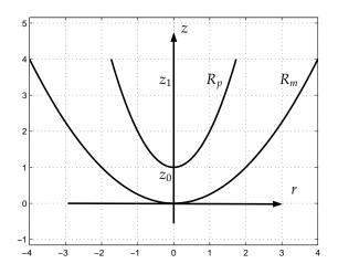
Figure 5.1: Mould and plunger geometries defined by parabolas.
