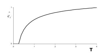
Figure 3. Breakthrough curves for unfavourable isotherms
