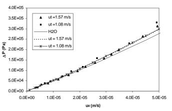
Figure 2 – Pressure drop vs membrane flux. The predictions are the solid lines whereas the experimental data are presented by the symbols.
