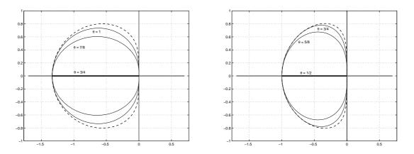
Fig. 3.2. Explicit stability regions  $S_0$  (dashed) and regions  $D_0$  for the IMEX BDF2 methods (left) and ADAMS2 methods (right).
