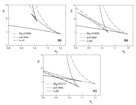
Figure 6 – Bifurcation sets obtained for *dc* model ( $\lambda$ =10,25,50), *d* model ( $\phi$ =0.7643) and *c* model (Da<sub>p</sub>=0.0584,0.0234,0.0117); (Da=0.0087,  $\gamma$ =21.8).
