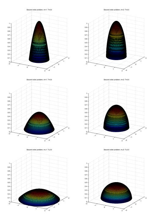
Figure 3: Snapshots of approximations to radially symmetric self-similar solutions (with corresponding triangular meshes) of the PME at three different times for m = 1,  $T = t - \frac{1}{8}$  (left) and m = 2,  $T = t - \frac{1}{6}$  (right).
