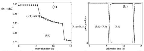
Fig. 3. Results for one batch. (a) specific growth rate estimates with a ME with 3 experts (9 parameters): measured values (0, dots), estimated values (-, solid line). (b) Gaussian gating network outputs:  $g_1$  (..., dot line),  $g_2$  (-, solid line) and  $g_3$  (--, dash line).
