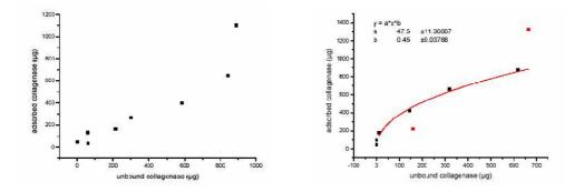
Figure 2: Adsorbtion of enzyme. Results after 3 hours (left) and 24 hours (right).
