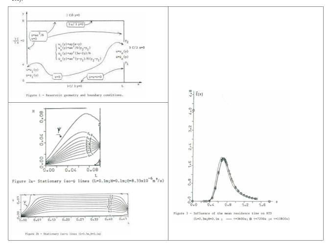
Figure 12. 2-D flow in a reservoir and RTD.
