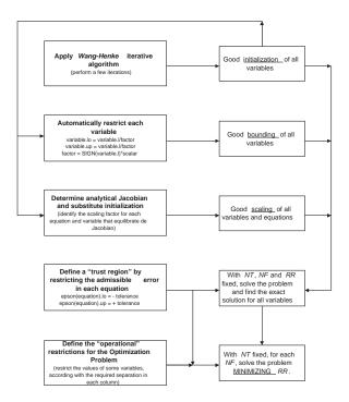
Figure 5: Schematic representation of the strategy for individual optimization of the distillation columns.
