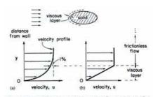
Fig. 1. Velocity profile near a wall: (a) actual profile, and (b) simplified profile.
