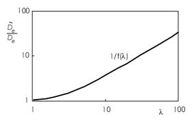
Figure 16. Enhancement factor for diffusivity due to convection,  $1/f(\lambda)$
