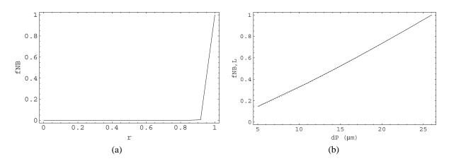
Figure 1: (a) intra-particular profile of MNB concentration, (b) dependence of the residual concentration of nitrobenzene with particle diameter. ).
