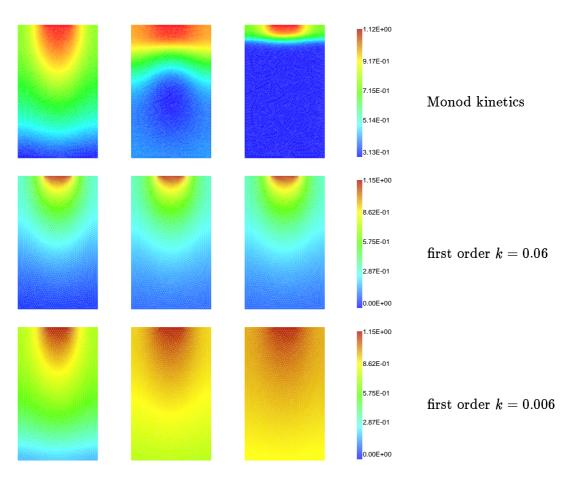
Figure 1: Simulation of benzene degradation with Monod kinetics (top), first order decay with k = 0.06 1/d (middle), and first order decay with k = 0.006 1/d (bottom) for t = 10 d (left column), t = 20 d (middle column) and t = 50 d (right column). Note the different ranges.
