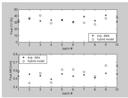
Fig. 6 Final CSD (CV and AM) - experimental data and hybrid model predictions
