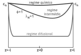
Figure 8. Assymetric concentration profiles in large pore catalysts
