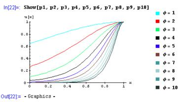
Figure 6 – Reactant concentration profiles for a first order reaction in a slab.
