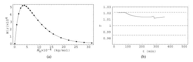
Figure 6: (a) Final PVC polymer molecular weight distribution and (b) the normalized optimal profile of the temperature polymerization (• obtained; – desired).
