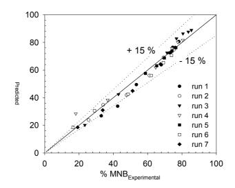
Figure 5 – Experimental versus predicted values of MNB concentrations in the organic phase outlet.
