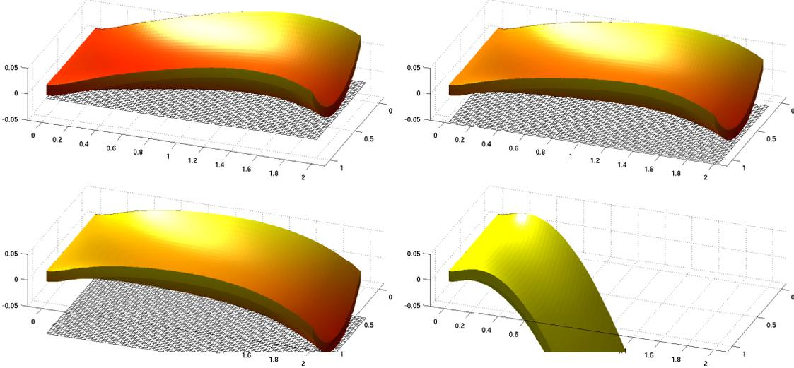
FIGURE 3. Example 2: Deformed plate for Example 1 with Coulomb friction, i.e.  $q = |\sigma_n|$ . Obstacle corresponding to  $s = 0.015$  (upper left), to  $s = 0.06$  (upper right), to  $s = 0.11$  (lower left) and deformation if not restricted with an obstacle (lower right). Note the small contact regions.
