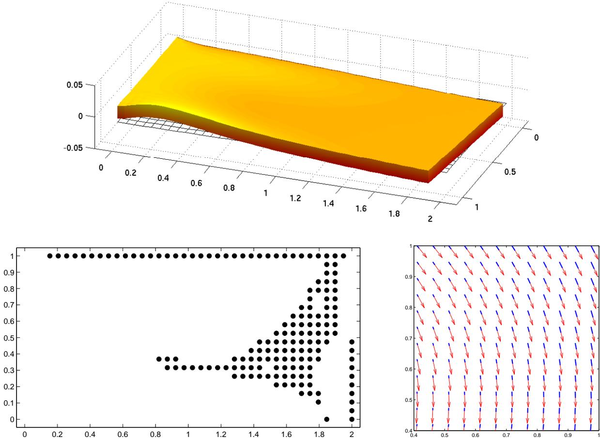
FIGURE 2. Example 1: Deformed plate (upper plot). Lower plots: nodes where the plate is in contact with the rigid obstacle (black dots in left plot); tangential displacement (blue lines in right plot) and tangential stress (red arrows in right plot) on a part of  $\omega$ .
