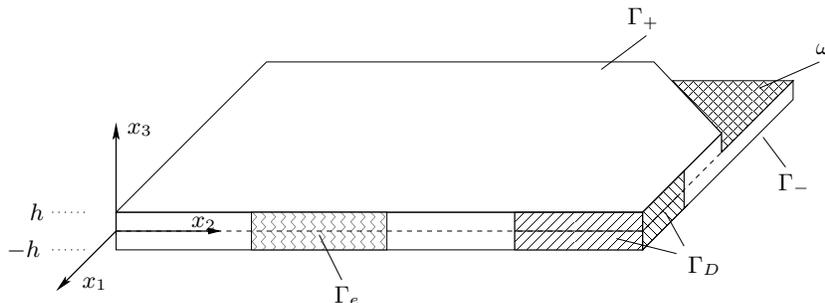
FIGURE 1. Three-dimensional plate  $\Omega$  with rectangular middle plane  $\omega$  and thickness  $2h$ .
