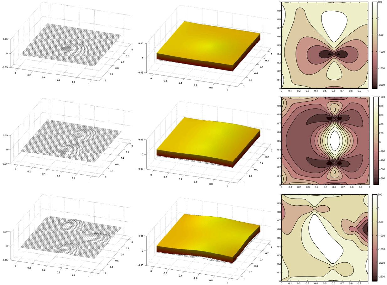
FIGURE 4. Example 3: Different obstacles (left row), the corresponding deformed plates (middle row) and contour plots of the electric potentials on  $\Gamma_+$ .
