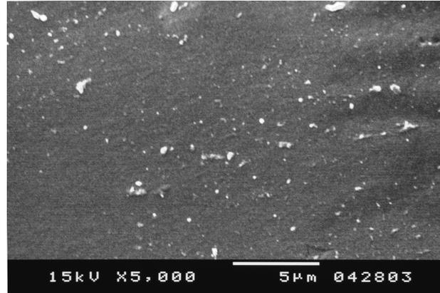
FIGURE 2. SEM image of the cross section of a copolymer with particles, at  $5000\times$  magnification.
