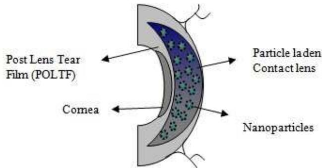
FIGURE 3. Schematic illustration of the ophthalmic lens inserted in the eye.
