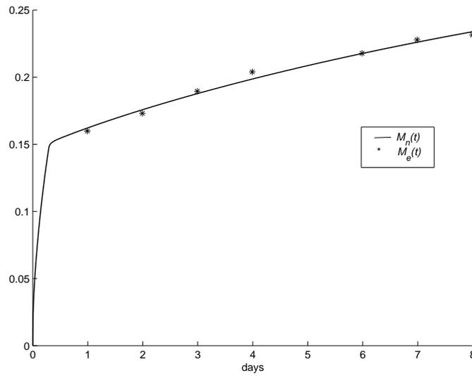
FIGURE 16. Numerical and experimental mass delivery from a contact lens with dispersed drug and entrapped particles loaded with drug during the first 8 days obtained with (45) and (42).
