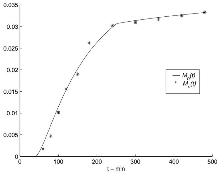
FIGURE 14. Numerical and experimental mass delivery from a lens with entrapped particles loaded with the drug during the first 9 hours obtained with (43) and (44).
