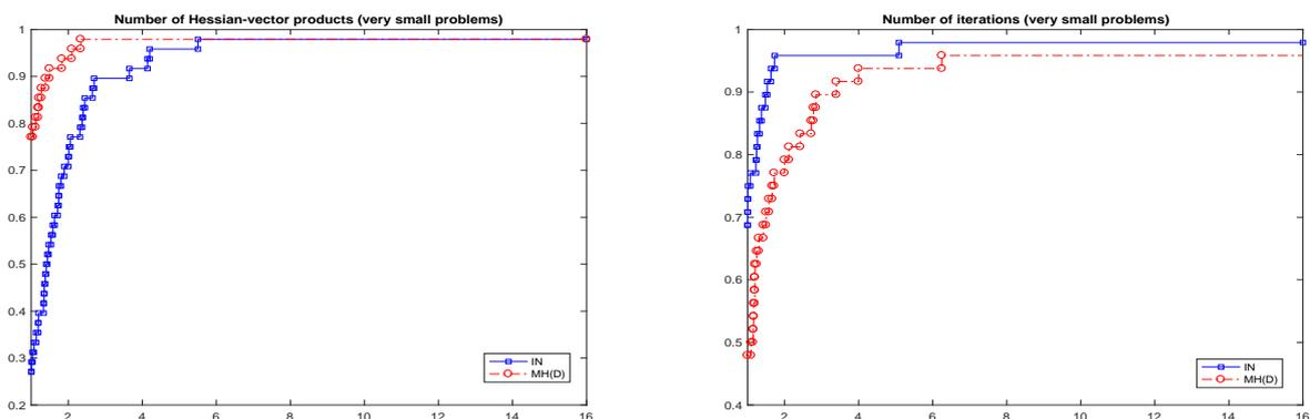
FIGURE 1. Testing the Hessian recovery within a line-search algorithm. Performance profiles for the numbers of Hessian-vector products and iterations, for the set of very small problems of Appendix B. The value of  $p$  was set to  $\frac{n^2+n}{2} - n$ .
