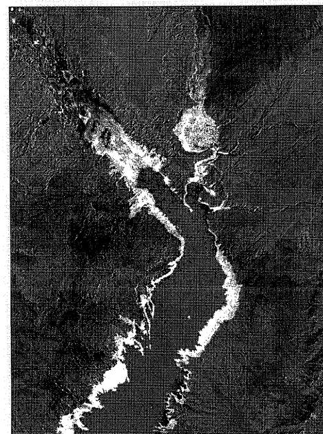
d. Image differencing change detection based on Landsat ETM + band 4 May 3, 2000 data and ASTER band 3 April 19, 2003 data.
