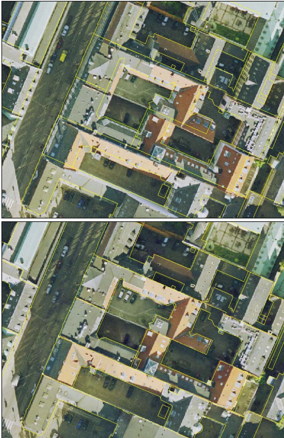
Figure 2.10 – Orthophoto (top) and true orthophoto (bottom) overlaid with a vector map of the building outlines. The orthophoto has a good fit with objects in level with the terrain, but not with objects like the rooftops that wasn't included in the rectification. With the true orthophoto this is not a problem.
