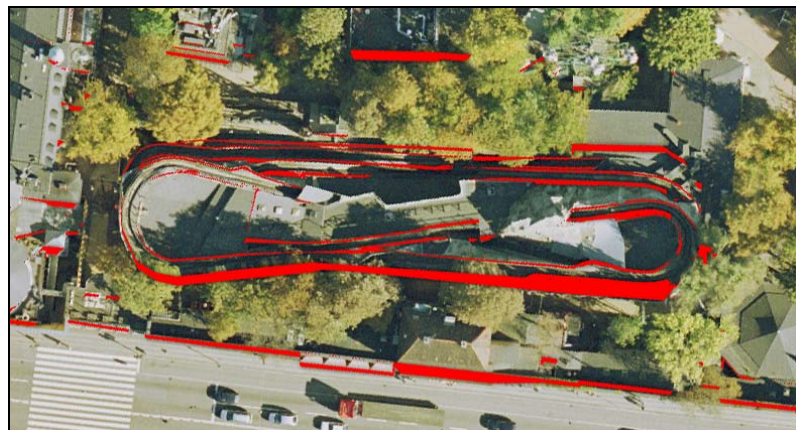
Figure 10.11 - Insufficient overlap causes many blindspots.
