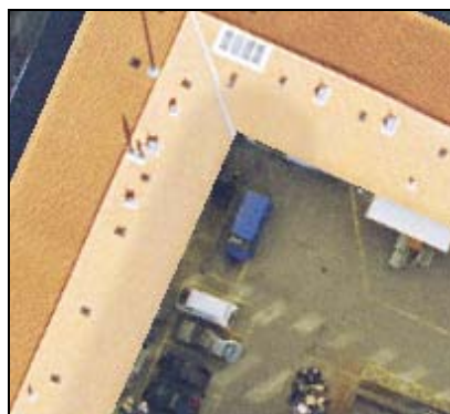
Figure 10.9 - Color match not perfect caused by light reflected differently in the source images.
