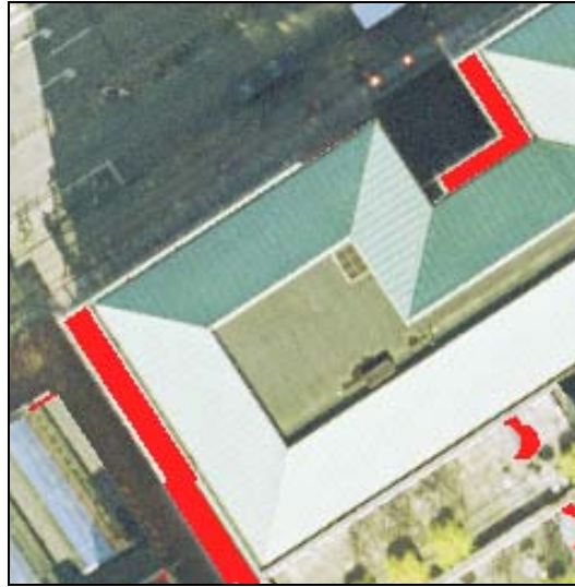
Figure 10.10 - Incorrectly detected blindspots caused by eaves missing in the DSM.
