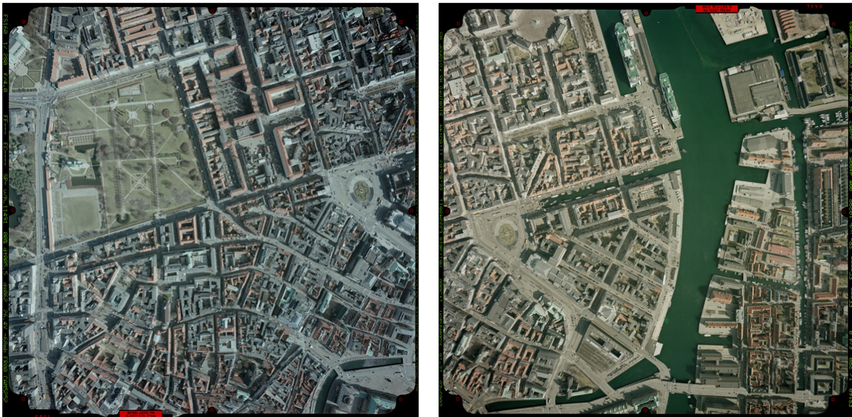
Figure 8.1 – Two neighboring images. The image on the left has a very bluish look compared to the image on the right. Since the original analog images doesn't have this color difference, it must originate from the scanning.
