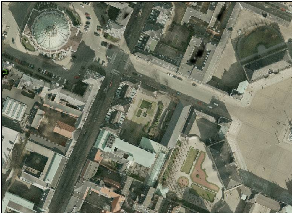
Figure 8.15 - Mosaic of histogram matched orthophotos. With a little feathering to smooth the edges, the seamlines are almost invisible.
