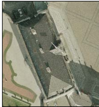
Figure 10.16 - Roof ridge not rectified to correct position.
