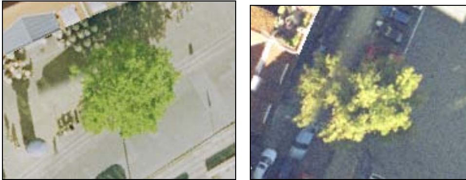
Figure 10.6 - Mosaicking of non-rectified trees is weird-looking, though hardly noticeable.
