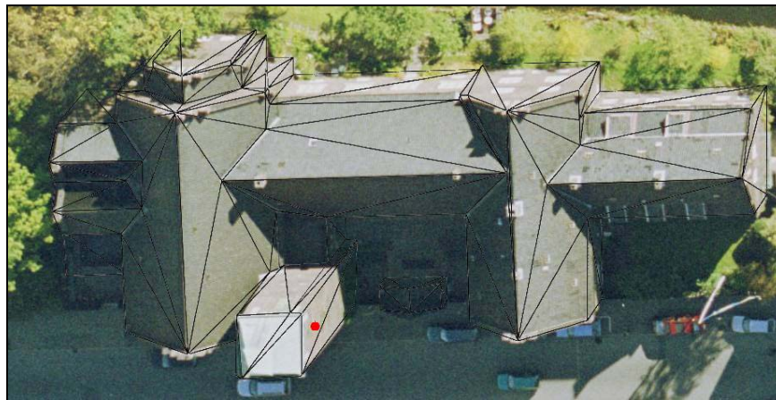
Figure 7.4 - Image of the same building as illustrated on the two previous figures. The transformed surface model has been superimposed.
