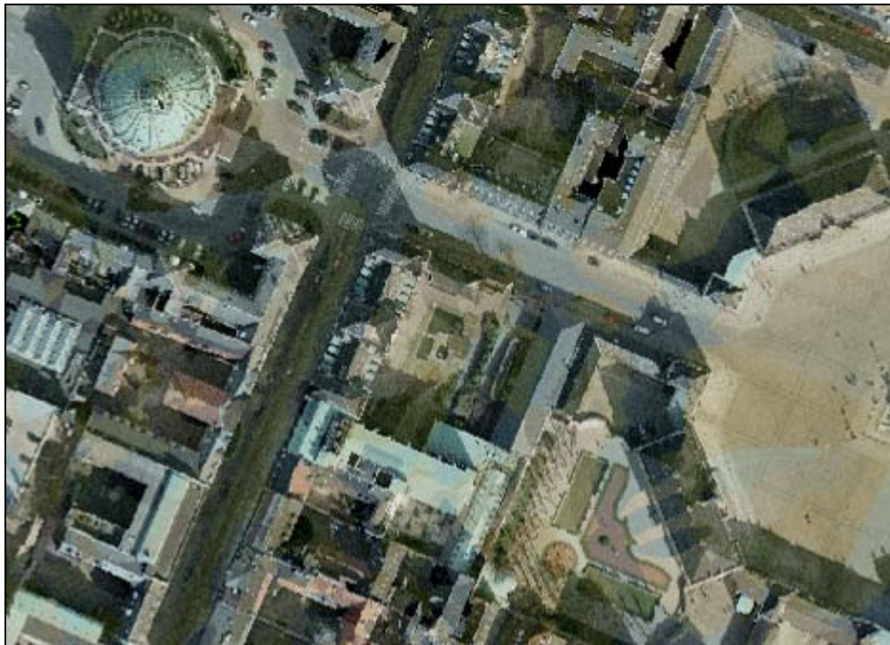
Figure 8.14 –True orthophoto mosaic. The original imagery are very different in color and intensity which causes a poor mosaic with very visible seamlines. Because of the big differences in color, feathering the seamlines isn't enough to hide the differences.
