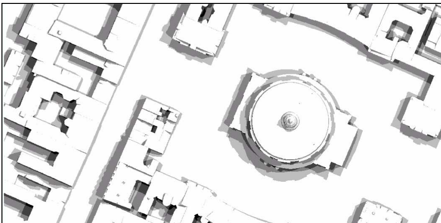
Figure 9.1 - Visibility analysis for four images. White is visible in all images, and black means obscured in all images. The three levels of gray specify that it is obscured in respectively 1, 2 or 3 images.
