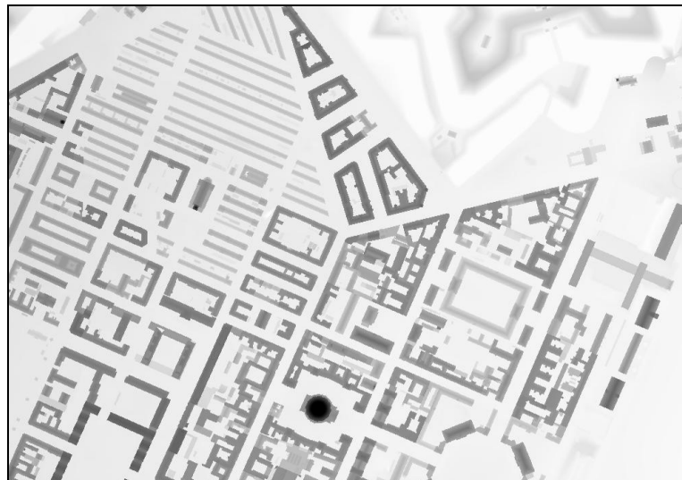
Figure 3.8 – Grid of a part of Copenhagen, where the intensity of each pixel corresponds to the height at the centre of the pixel. A low intensity (dark) represents taller buildings. The grid is created from a TIN by sampling pixel by pixel.
