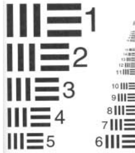
Figure 2.15: Typical test pattern (three-bar target) for determining resolving power.
