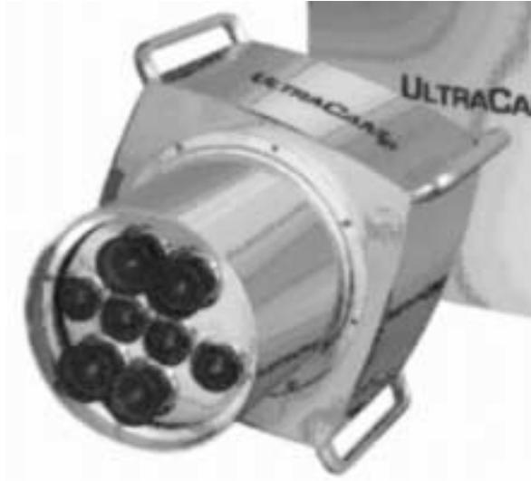
Figure 3.3: Example of a multi-camera system (Vexcel UltraCam), consisting of 8 different cameras that are mounted in a slightly convergent mode to assure overlap of the individual images.
