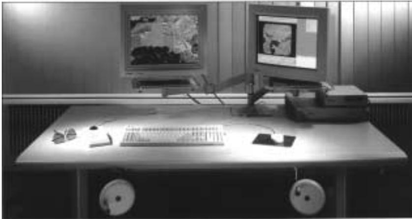
Figure 6.8: Typical digital photogrammetric workstation. The system shown here offers optional handwheels to emulate operation on classical photogrammetric plotters. Courtesy LH Systems, Inc., San Diego, CA.
