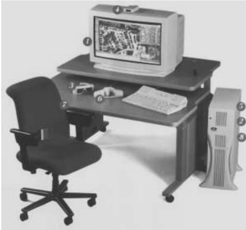
Figure 6.9: Digital photogrammetric workstation. Shown is Intergraph's ImageStation Z. Main characteristic is the large stereo display of the 28-inch panoramic monitor. Courtesy Intergraph Corporation, Huntsville, AL.
