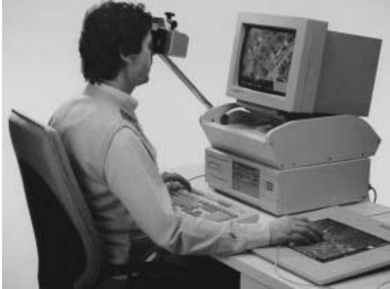
Figure 6.12: Example of a split-screen viewing system. Shown is the DVP digital photogrammetric workstation. Courtesy of DVP Geomatics, Inc., Quebec.
