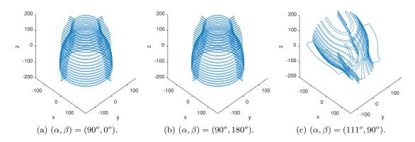
Figure 5: Duct object slices at optimal rotations.
