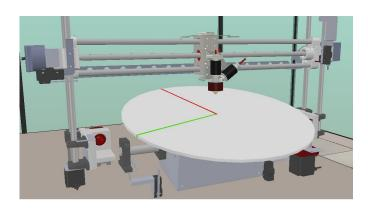
Figure 1: Virtual representation of the 5-axis printer (FIBR3DEmul [9]).
